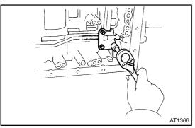
7. INSTALL PARKING LOCK PAWL BRACKET Torque: 7.4 N-m (75 kgf-cm, 65 in.-lbf)
