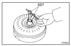
(b) Install SST so that it fits in the notch of the converter hub and outer race of the one–way clutch.
