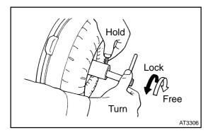
(c) With the torque converter clutch standing on its side, check that the clutch locks when turned counterclockwise, and rotates freely and smoothly clockwise.
