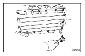
(e) Install the oil pan with the 19 bolts.
