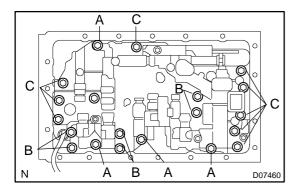
(b) Install the valve body with the 20 bolts.
