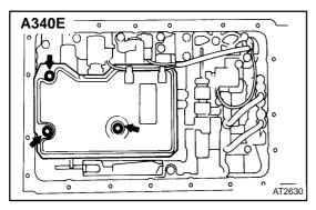
(b) Install the oil strainer with the 3 bolts.
