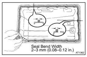
(c) Remove any packing material and be careful not to drop oil on the contacting surfaces of the transmission case and oil pan.
