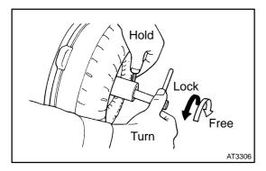
(c) With the torque converter clutch held upright, the clutch should lock when turned counterclockwise, and rotate freely and smoothly clockwise.
