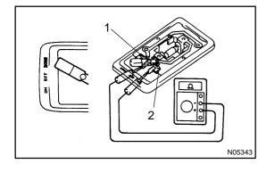
(c) Turn the room light switch to DOOR, check that there is continuity between terminals 1 and 2.
