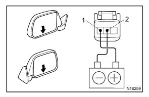
(d) Reverse the polarity, check that the mirror turns downward.
