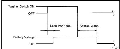
If operation is not as specified, replace the wiper and washer switch.
