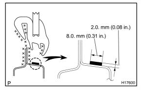
(b) Apply soapy water to the contact surface of the body and the weatherstrip lip.
