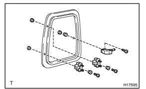
(b) Remove the lock handle from the quarter window glass.(c) Remove the 2 hinges from the quarter window glass.
