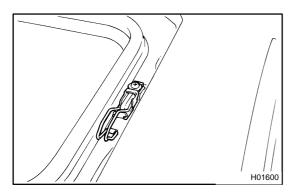
**4. REMOVE REMOVABLE ROOF AUXILIARY CATCH** Remove the screw and auxiliary catch.
