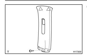
(e) Using a screwdriver, remove the screw, upper center pillar garnish.
