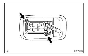
(b) Remove the 2 screws, and room lamp, disconnect the connector.
