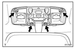
(b) Remove the 4 screws, map lamp and mirror, disconnect the connector.
