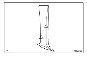
(d) Using a screwdriver, remove the lower center pillar garnish.
