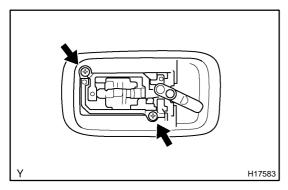
(b) Remove the 2 screws and room light, then disconnect the connecter.
