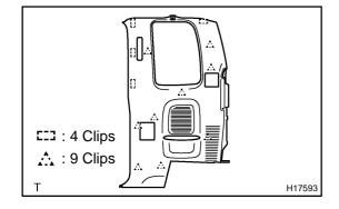
(g) Using a screwdriver, pry and remove the quarter trim.
