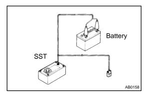
Check functioning of SST. (b) (See step 1-(a)) 09082-00700, 09082-00770 SST
