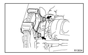
(f) Install the torque plate onto the knuckle.
