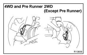
(c) Remove the speed sensor installation bolt from the steering knuckle.
