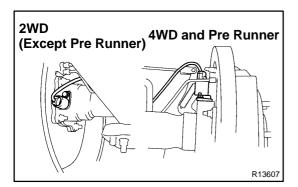
(c) Remove the 2 mounting bolts and speed sensor.
