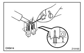
(c) Solder the brush wire to the brush holder at the specified exposed length.
