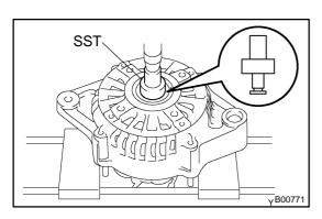
(b) Using SST and a press, press out the bearing. SST 09950–60010 (09951–00260, 09952–06010)
