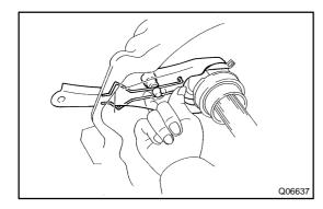
(c) Remove the set bolts, and pull off the clutch cover with the clutch disc.
