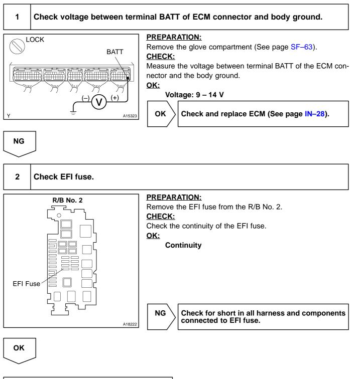
Check and repair harness or connector between battery and EFI fuse, and EFI fuse and ECM.
