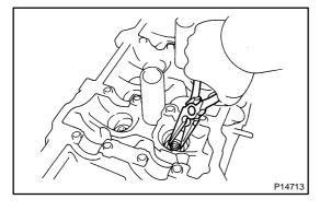
(c) Using needle-nose pliers, remove the oil seal.
