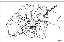
(d) Using compressed air and a magnetic finger, remove the spring seat by blowing air.
