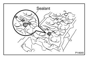
(b) Apply adhesive to the spark plug tube hole of the cylinder head
