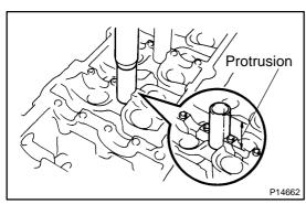
(c) Using a press, press in a new spark plug tube until there is 47.0 mm (1.850 in.) protruding from the camshaft bearing cap installation surface of the cylinder head.
