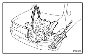
(b) Attach the engine hoist chain to the 2 engine hangers.
