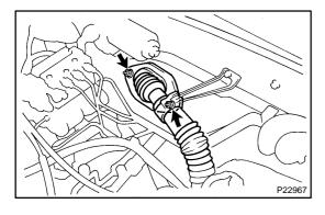
(g) Remove 2 nuts holding the engine wire retainer to the cowl panel and pull out the engine wire from the cabin.
