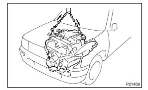
Lift the engine with transmission out of the vehicle slowly (e) and carefully.
