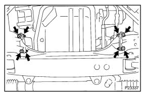
(d) Remove the 4 bolts and 4 nuts holding the engine front mounting insulators to the frame.
