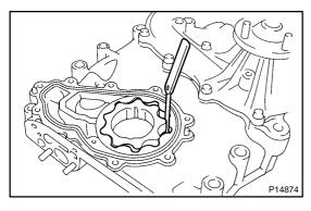
(c) Inspect the rotors for side clearance.
