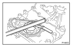
(b) Inspect the rotors for tip clearance.
