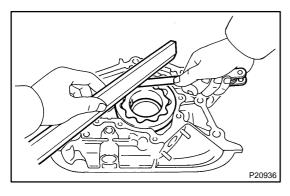
(c) Inspect the rotors for side clearance.
