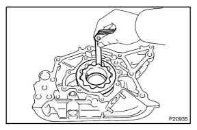
(b) Inspect the rotors for tip clearance.
