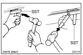
(b) Using SST and a brass bar, separate the oil pan from the cylinder block.
