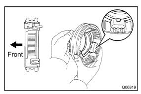
(g) While pushing the 3 shifting keys, install the synchronizer ring assembly to the hub sleeve No.3.
