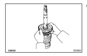
(d) Install the assembly on the output shaft with the synchronizer ring slots aligned with the shifting keys.
