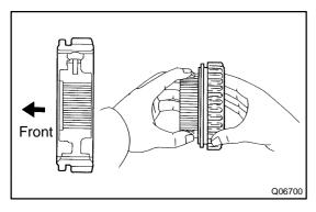
(c) While pushing the 3 shifting keys, install the clutch hub No.1 to the reverse gear, as shown.
