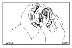
3. INSTALL 3RD GEAR AND HUB SLEEVE NO.2 ON OUTPUT SHAFT
