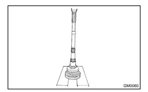
(d) Using a press, install the 3rd gear and hub sleeve No.2.
