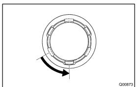
(d) Turn the reverse synchronizer pull ring and separate the pull ring and cone ring.
