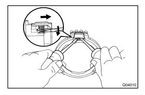
(e) Remove the 3 shifting keys and key springs by carefully levering up the shifting key spring with one screwdriver and levering the shifting key away from the reverse synchronizer ring with another screwdriver.
