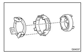
(c) Remove the reverse synchronizer ring and 5th synchronizer ring from the synchronizer pull ring and cone ring.
