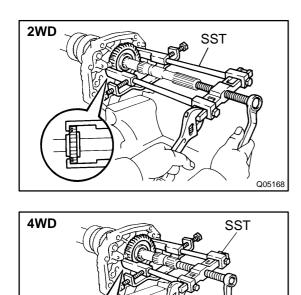
(b) Using SST, remove the reverse gear. SST 09950–40011
