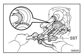
(b) Using SST, remove the rear bearing, spacer, 5th gear and bearing.
