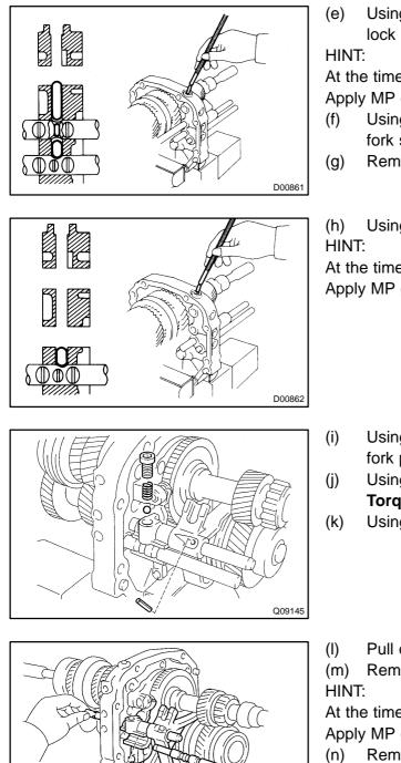
e) Using a magnetic finger, remove the No.1 and No.2 interlock pins.
