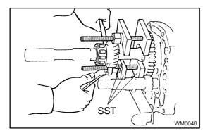
(b) Using SST, remove the rear bearing and 5th gear. SST 09312–20011 (09313–00030, 09313–00040, 09313–00050)
