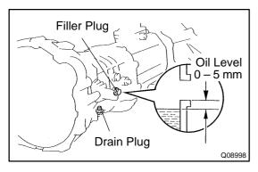
3. RAISE VEHICLE AND DRAIN TRANSMISSION OIL
