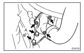
(c) Remove the 2 set bolts of the front exhaust pipe bracket. **Torque:**
