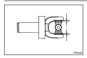
(e) Using SST, adjust both bearings so that the snap ring grooves are at maximum and equal widths.
