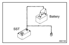
Connect the SST to the battery.
