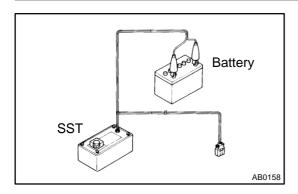
(c) Confirm functioning of the SST. SST 09082–00700
