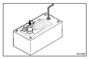
(2) Confirm functioning of the SST. Press the SST activation switch, and confirm the LED of the SST activation switch lights up.
