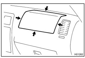
There should be no interference between the instrument panel and front passenger airbag door, or the glove compartment door and front passenger airbag door. The clearance should be uniform all the way around when the new airbag assembly is installed on the instrument panel.
