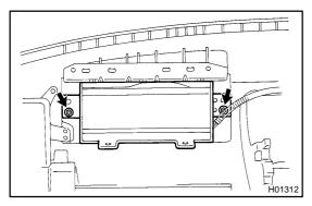
(b) Install the front passenger airbag assembly to the instrument panel.
