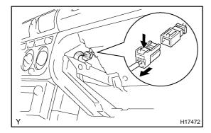
(c) Disconnect the airbag connector.
