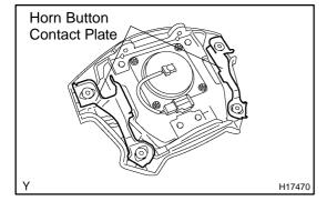
• Check the deformation of the horn button contact plate on the steering wheel pad.
