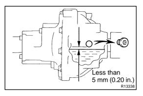
FILL DIFFERENTIAL WITH HYPOID GEAR OIL Torque: 39 N·m (400 kgf·cm, 29 ft·lbf) Oil type: Hypoid gear oil API GL-5 Recommended oil viscosity: SAE 75W-90 Capacity: 1.15 liters (1.22 US qts, 1.01 lmp. qts)
