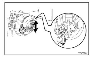
(b) Using a dial indicator, check the lower ball joint for excessive play when you push the hub nuts up and down with a force of 294 N (30 kgf, 66 lbf).
