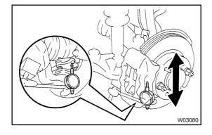
(b) Using a dial indicator, check the lower ball joint for excessive play when you push the hub nuts up and down with a force of 294 N (30 kgf, 66 lbf).
