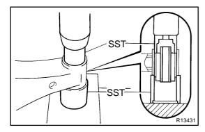
(b) Face the cut side downward and using SST and a press, remove the bushing.
