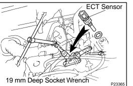
(c) Using a 19 mm deep socket wrench, remove the ECT sensor and gasket.
