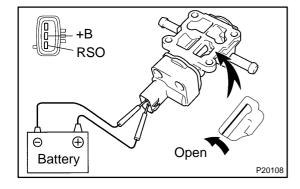
(b) Connect the positive (+) lead from the battery to terminal +B and negative (-) lead to terminal RSO, and check that the valve is open.
