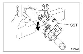
(b) Using a spanner to hold the steering rack steady, and using SST, remove the rack end.
