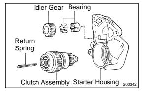
(b) Remove the starter housing, return spring, the clutch assembly, idler gear and bearing from the magnetic switch assembly.
