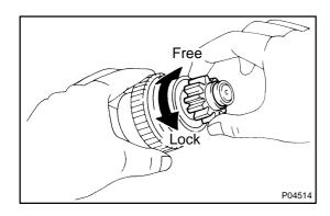
(b) Check the clutch pinion gear.
