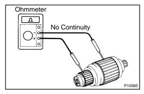
(b) Check the commutator for ground.Using an ohmmeter, check that there is no continuity between the commutator and armature coil core.
