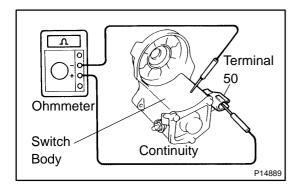
(b) Check the hold-in coil for open circuit.Using an ohmmeter, check that there is continuity between terminal 50 and the switch body.
