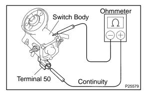
(b) Check the hold-in coil for open circuit.Using an ohmmeter, check that there is continuity between terminal 50 and the switch body.
