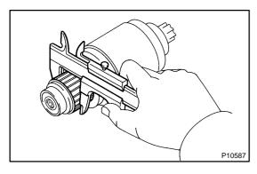
(c) Using vernier calipers, measure the commutator diameter.
