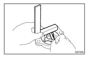
(f) Inspect the both rotors side clearance.
