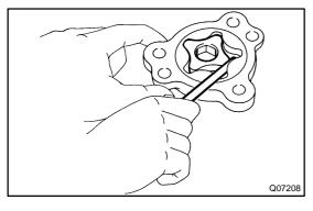
(e) Inspect the both rotor tips clearance.
