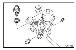
(c) Remove the O-ring, 4WD position switch and snap ring from the actuator assembly.
