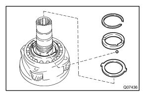
(b) Remove the input gear stopper, thrust washer and ball. HINT:
