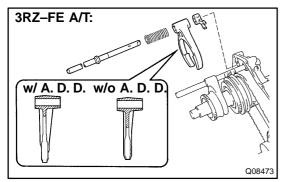
(d) Remove the front drive fork shaft, shift fork, spring and stopper.
