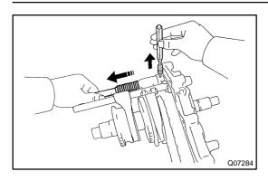
(c) Hold the front drive fork shaft in place by hand, when removing the pin punch.
