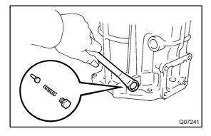
(b) Remove the plug, spring and pin.
