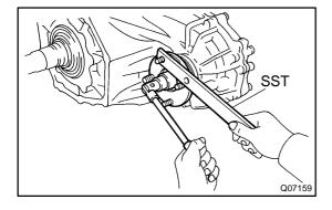
(b) Using SST to hold the flange, remove the companion flange lock nut.
