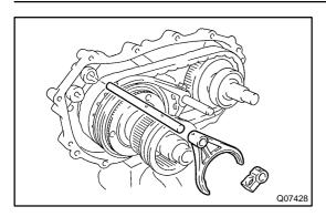
(c) Remove high and low fork shaft, shift fork and shift gear head No.2.
