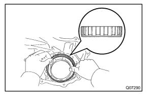
(c) Remove the planetary ring gear.
