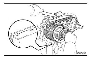
(c) Using a plastic hammer, tap the rear case with pulling the rear output shaft, driven sprocket and front drive shift fork.
