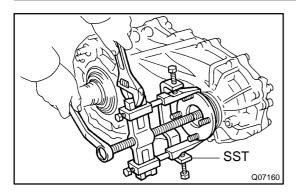
(c) Using SST, remove the companion flange. SST 09950-40011 (09951-04020, 09952-04010, 09953-04030, 09954-04010, 09955-04051, 09957-04010, 09958-04011)
