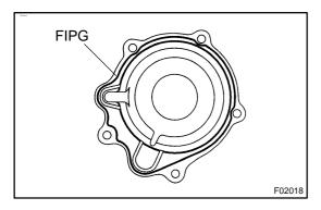
(b) Using a plastic hammer, tap the front bearing retainer and remove it.
