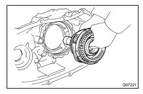
(b) Pull out the planetary gear assembly with the input shaft. HINT:
