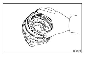
(b) Remove the low gear spline piece.
