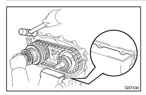
(b) Using a plastic hammer, tap the rear case with pulling the rear output shaft and driven sprocket.
