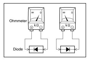
If the circuit has diodes, reverse the two leads and check again.
